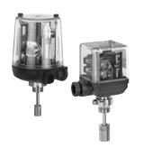
The GEMÜ 1211 and 1231 electrical position indicators have one or two proximity switches for end position feedback which are mechanically adjustable. The devices are suitable for installation in Ex-proof applications acc. to ATEX. GEMÜ 1211 is suitable for mounting to linear actuators with a max. stroke of 70 mm. GEMÜ 1231 is suitable for mounting to linear actuators with a max. stroke of 20 mm.
