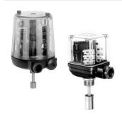
The GEMÜ 1201 and 1230 electrical position indicators have one or two microswitches for end position feedback which are mechanically adjustable. GEMÜ 1201 is suitable for mounting to linear actuators with a max. stroke of 70 mm. GEMÜ 1230 is suitable for mounting to linear actuators with a max. stroke of 20 mm.
