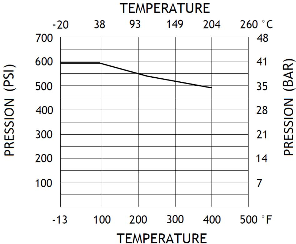
**CLAPET DE NON RETOUR WAFER A DISQUE INOX TOUTES POSITIONS PN40**
